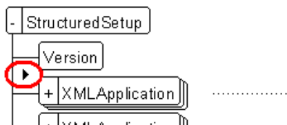
Figure 2-1: Structure View window insertion point
